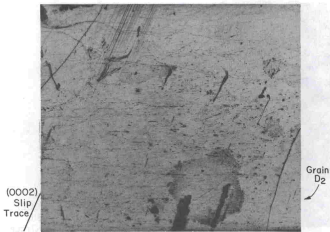
Fig. 4—Grain E_2 sample Zn-15 after exposure to 11.86 kbars. Polarized light; X48. Reduced approximately 47 pct for reproduction.
